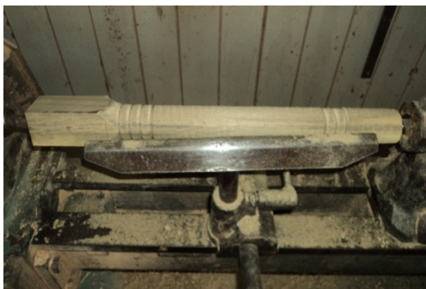
Figure 1. X. pacifica work piece under turning and moulding process into a coffee table leg in the lathe machine.
